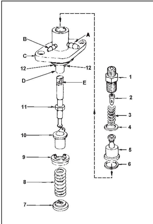
**Injection pump components and disassembly**
