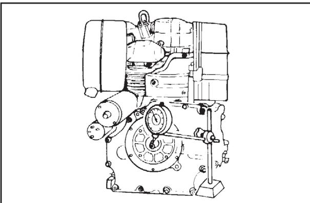
Secure the engine to a metal base or table. Use a dial indicator with column and magnetic base plate. Place the stylus on the crankshaft.
