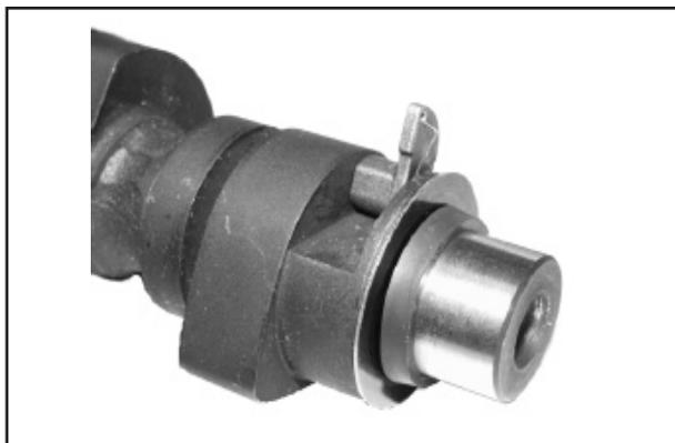
During normal operation, the tappet overcomes the spring resistance while passing on the system and decompression does not operate.
