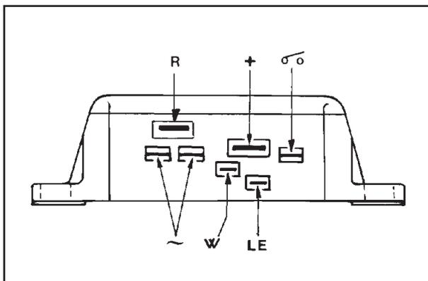
12V, 12A: for standard alternators with 3 output wires
