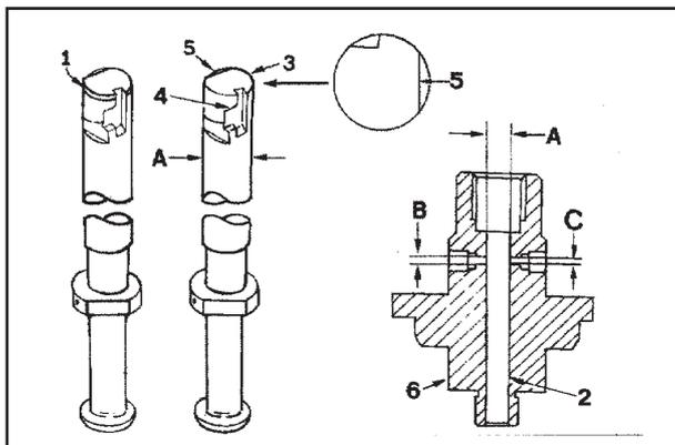
**Injection pump, body, plunger and delivery valve**
