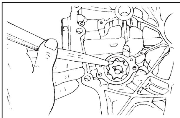
**Oil pump - Clearance between rotors**
