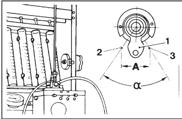
**Injection pump delivery check on test bench**
