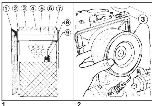
**!** Clean the filtering element with air blast. Air must be blown from inside to outside the cartridge at a distance of at least 15 cm from the paper. Lightly and repeatedly tap the element on a hard surface to eliminate all excess dirt.
