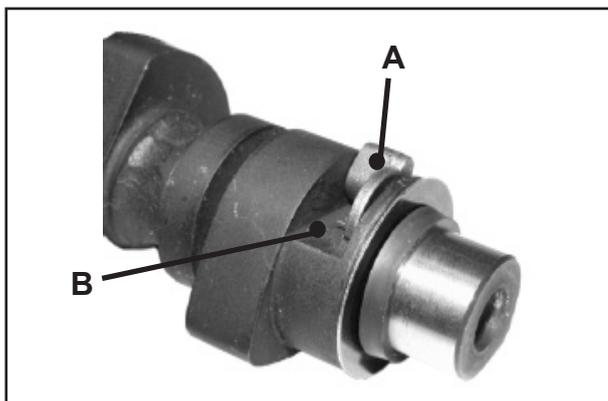
In case of a startup in reverse direction, the antireverse system lifts the valve as the tappet passes by. Startup is thus inhibited.
