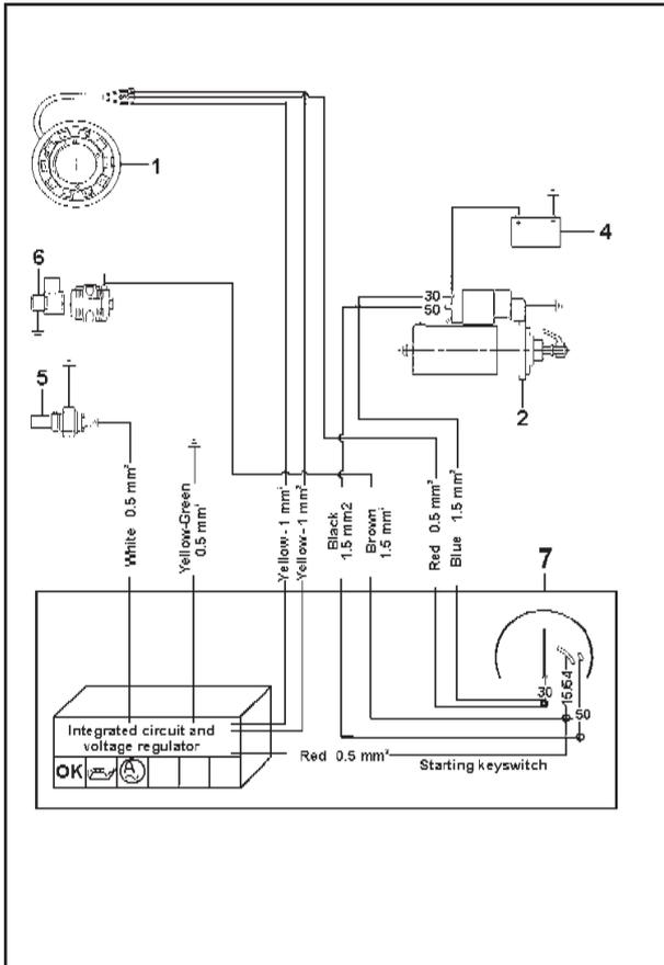
**12V electric starter diagram with voltage regulator built into the ignition panel**
